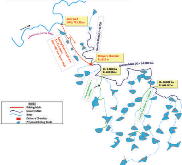
Scheme to lift water from Lakshmanateertha River near Mardur Village to fill 47 Tanks in Hunsur Taluk & 2 Tanks in H.D. Kote Taluk of Mysore District.
